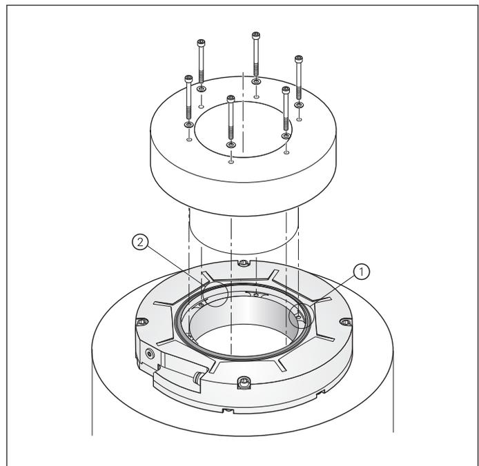
Example of shaft connection at encoder face
