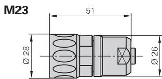
**Coupling insulated:** Connecting element with external thread; available with male or female contacts.
