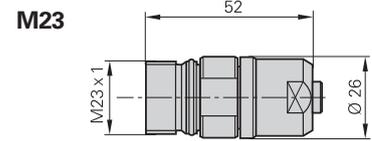
**Mounted coupling with central fastening**
