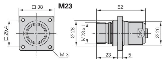
**Flange socket:** Permanently mounted on the encoder or a housing, with external thread (like a coupling), available with male or female contacts.
