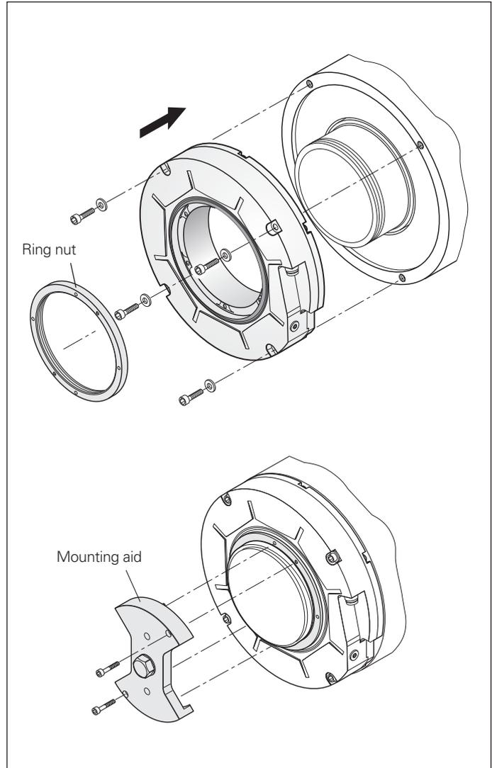
Mounting an angle encoder with hollow through shaft
